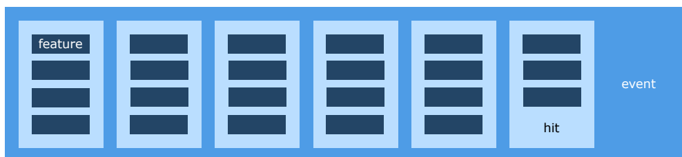
Figure 2. Data representation diagram, where dark blue rectangles represent features and light blue ones hits in the event sequence.
