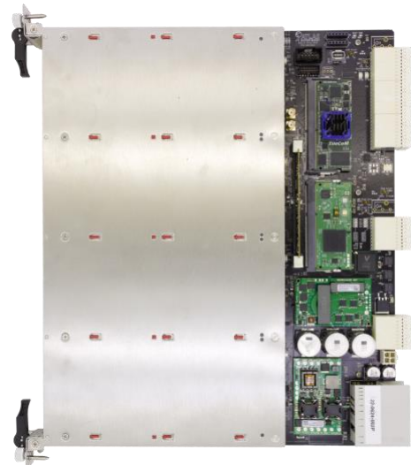
Fig. 10 ACBB board, including the TileCoM, IPMC and TileGbE switch mezzanine boards.
