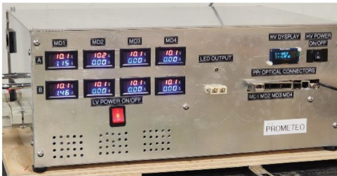
Fig. 15 PROMETEO box with all the connections for module certification.
