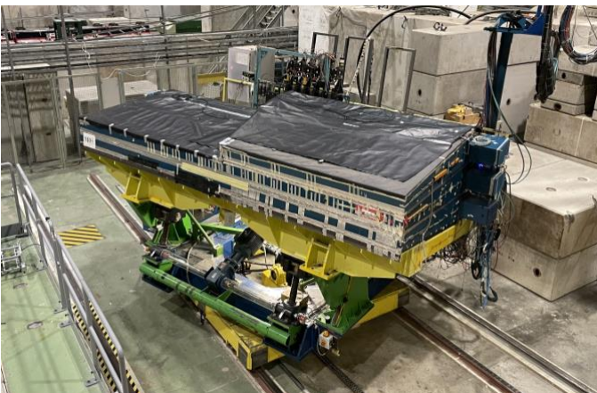
Fig. 16 TileCal test beam modules at the H8 beam line of the CERN SPS North Area.
