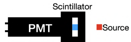
Fig. 5: Experimental setup for gamma-ray detection with 5x5x5 mm EJ-276D scintillator coupled to a PMT (1.3 kV) in front of a 125 kBq 137 Cs source.
