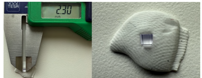
Fig. 2: Size of the first cut of EJ-276D scintillator (left), and picture of the modeling clay use to hold the piece in place for further cutting (right).
