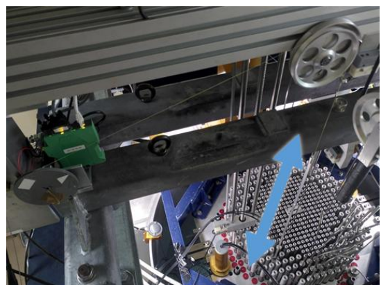
Fig. 2. The POLLEN pile-oscillator installed in the CROCUS zero-power reactor. On the left, motor, controller and wheel. The wire passes through the control rod pulley (on the top right) for precision guiding. The ruler connected to the wire is visible next to the double arrow that illustrates the linear displacement. The bottom of the ruler is inserted in the channel, with exiting optical fibers connected to miniature detectors set at the irradiation location.
