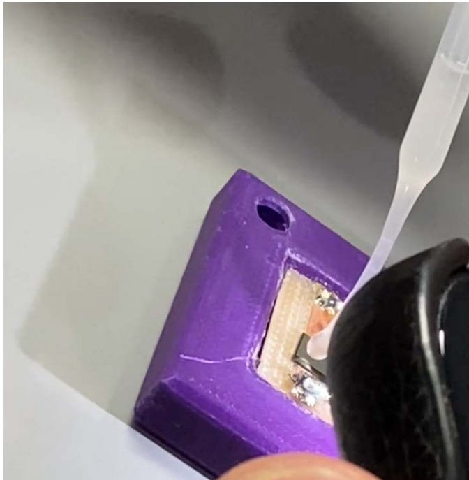
Fig. 1. Deposition of one drop of ^6\text{LiF} ethanol solution onto the surface of a SiC diode.
