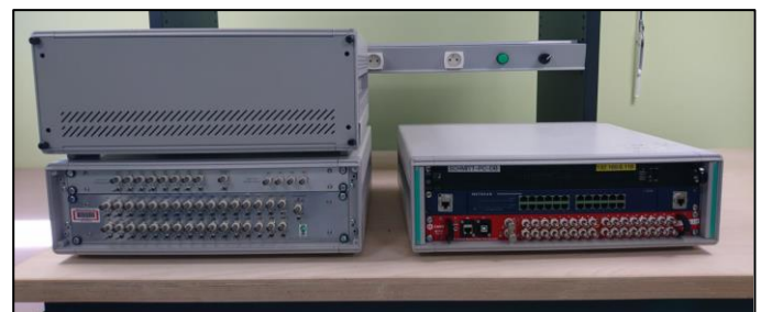
Figure 1. The legacy X-MODE DAQ on the left and new SCHMITT DAQ on the right.
