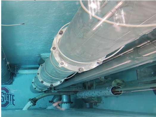
Fig. 1. Picture of the OSU research reactor, with a 23.7 cm diameter dry channel installed against the core casing.
