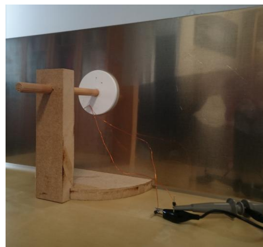
Fig. 4. Measurement of magnetic field attenuation through a 4 mm slab of aluminum.
