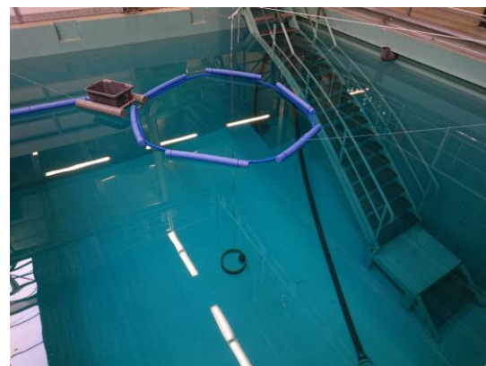
Fig. 3. General set-up for underwater testing. The transmitter antenna is located close to the basin floor, and the receiver antenna is floating on top.
