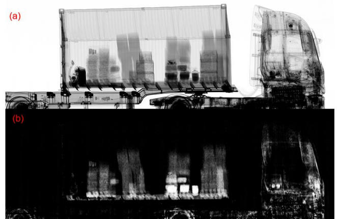
Fig. 5. Transmission image (a) and Wall Removal image (b) of the same truck.
