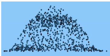
Figure 12: Image shows the top 20% of particles based on diameter for the simulation with 0.045 J/m^2 of adhesion.
