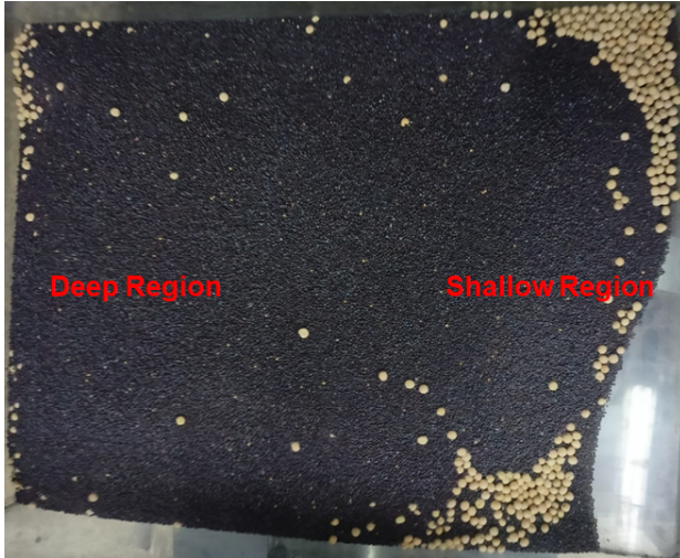
Figure 3: Initially, the pale yellow coloured boulders are distributed randomly in the black coloured grain bed. The above figure shows a top view of the final state after oscillating the box for a long time. Most boulders accumulate in the shallow region. The direction of oscillation is normal to the image.
