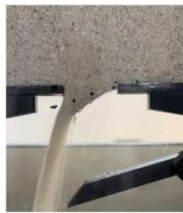
Fig. 3. Picture of the granular flow limited by the elastic gate.
