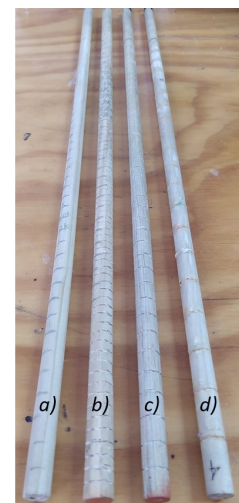
Figure 2. Rods used in the experiments. Left to right: a) smooth rod. Rods with grooves every: b) 0.5 cm, c) 1 cm, d) 1.5 cm.
