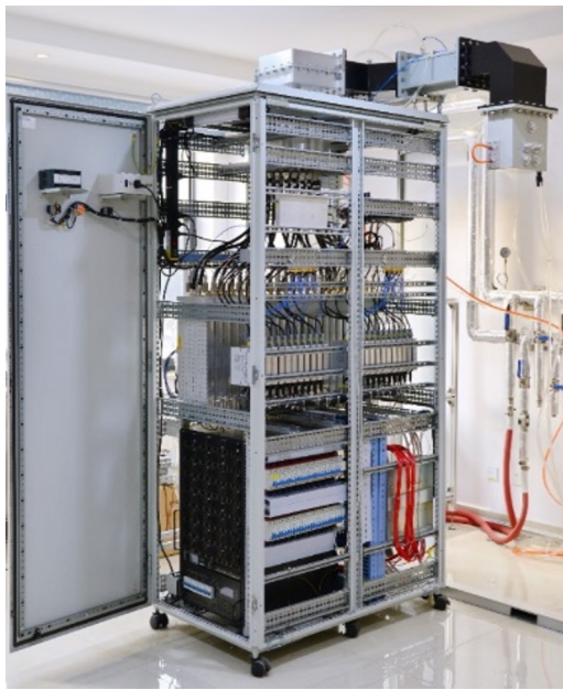
Fig. 11. Engineering prototype implementation of 20 kW solid-state microwave source.
