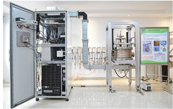
Fig. 13. 20 kW solid-state MPCVD system @ 915 MHz.
