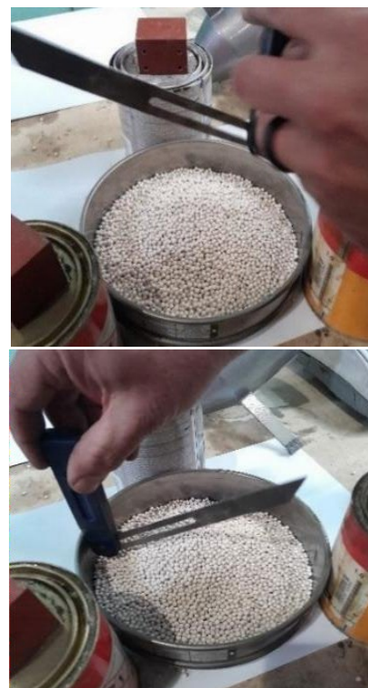
Fig 1. Angle of repose experiment (source: Drytech International (Pty) Ltd)
