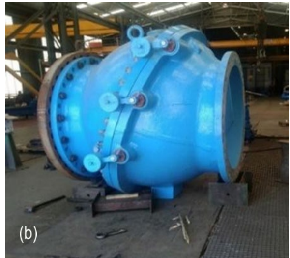
Fig. 1. Non-return multi-door reflux valve (a) schematic multi-door valve (1)-Inspection cover, (2)-Door's lever arm & counterweights, (3)-Outlet body, (4)- Door's main spindle (b) Physical valve.
