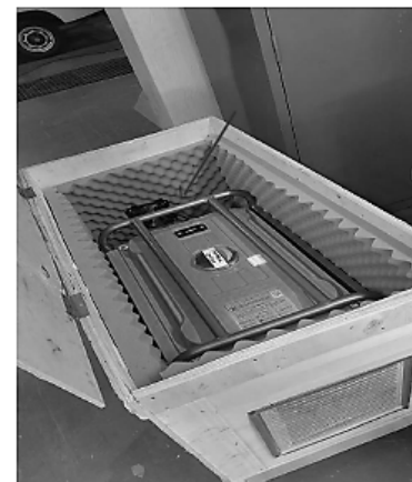
Fig. 13. Enclosed noise insulator
