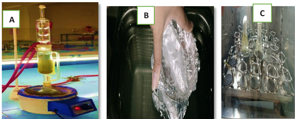
Fig. 2. Extraction process by A-Soxhlet process, B) Evaporation process, C) Maceration method
