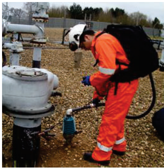
Fig. 1. High-Flow sampler measuring a leak rate.
