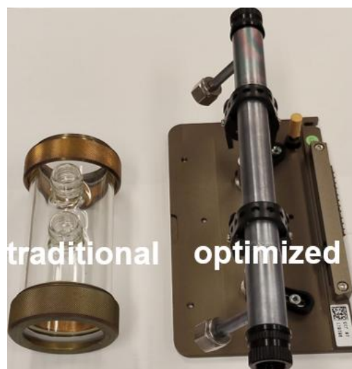
Figure 1 Single-pass cells for FTIR measurements. The cell on the left is a traditional 10 cm cell, with a relatively large volume. The cell on the right has been optimised for the analysis of reactive gases by minimizing the cell volume and use of SilcoNert 2000 passivation.
