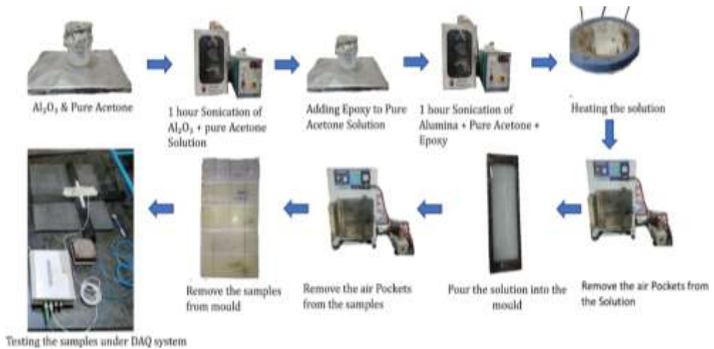
Fig. 3.1 Experimental procedure for determining dynamic and shear properties of epoxy- Al 2 O 3 composites as per ASTM E1876, including specimen preparation, support arrangement, and measurement of resonance frequencies for modulus calculation.
