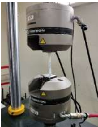
Fig. 1.2 Tensile testing setup for epoxy- Al 2 O 3 composite and Tensile test specimen prepared as per ASTM D638
