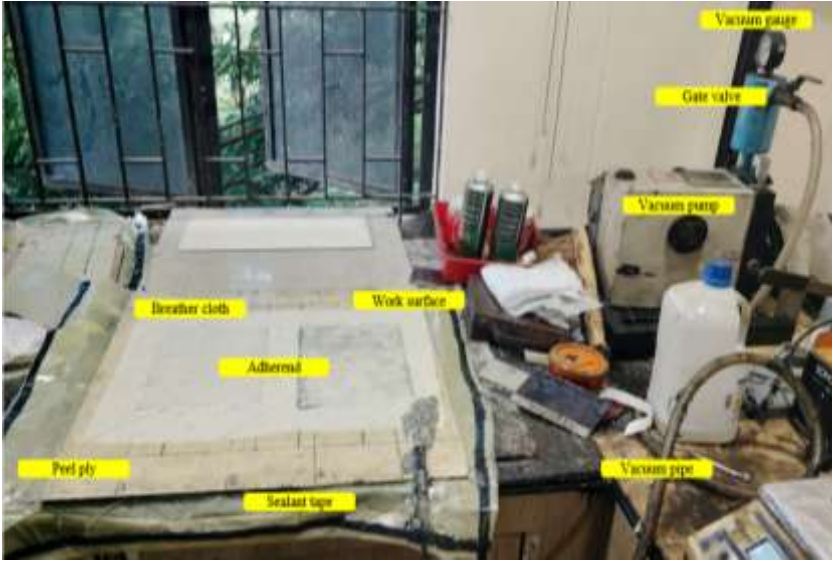
Fig. 4. Vacuum bagging setup for composite plate fabrication
