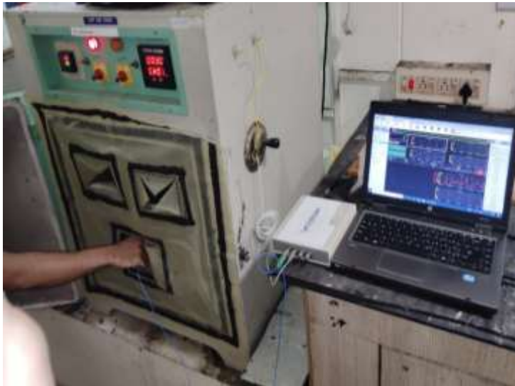
Fig. 11. Experimental setup for Modal vibration analysis using an FFT analyser
