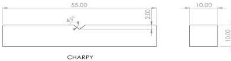
Fig 2) Specimen dimensions for Charpy V-notch impact test
