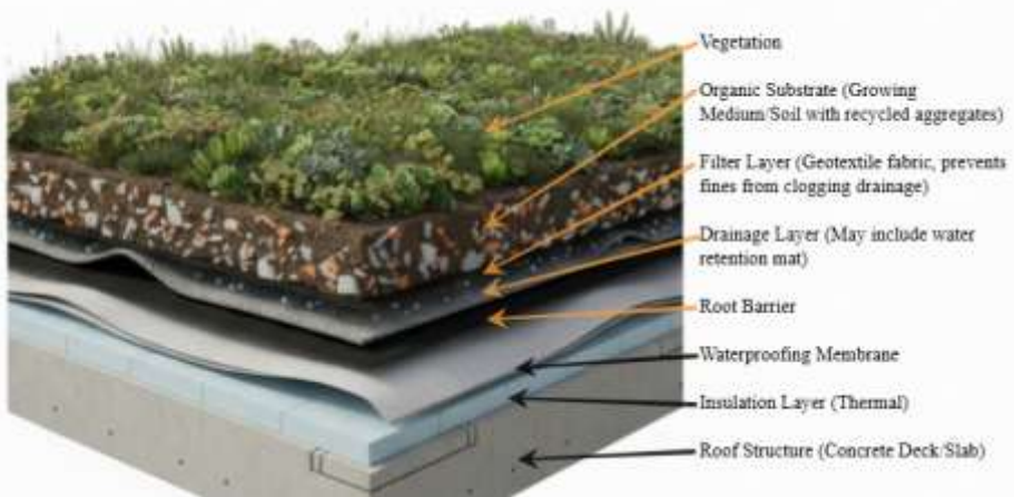
Fig. 1. Standard green-roof assembly with vegetation, growing media (substrate), filter/drainage layer, root barrier, waterproofing membrane, insulation, and roof frame structure.
