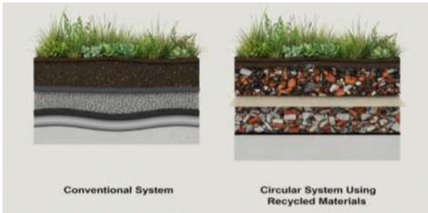
Fig. 3. A representative illustration of the Cross-section and experimental layout of green-roof prototypes built with recycled/reused materials.
