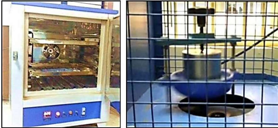
Fig 3 (a) Preheating CSA Powders on Furnace (b) Blending and sizing of powders in Ball Mill
