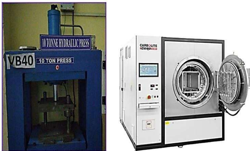
Fig 4. (a) Compacting of Specimens in Hydraulic Press (b) Sintering of specimens in Box Furnace
