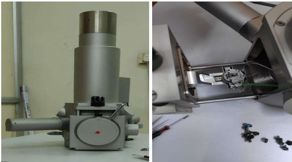
Fig 7. a) Scanning Electron Microscopy b) sample loading on the SEM
