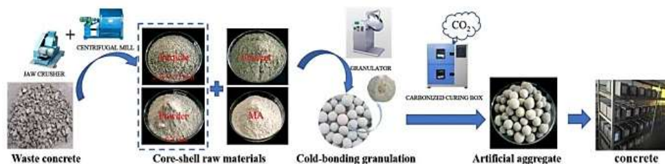
Fig. 2 Process of making artificial aggregates
