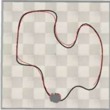
Fig. 8. Robot path on the training circuit with a 7x7 Q-table.
