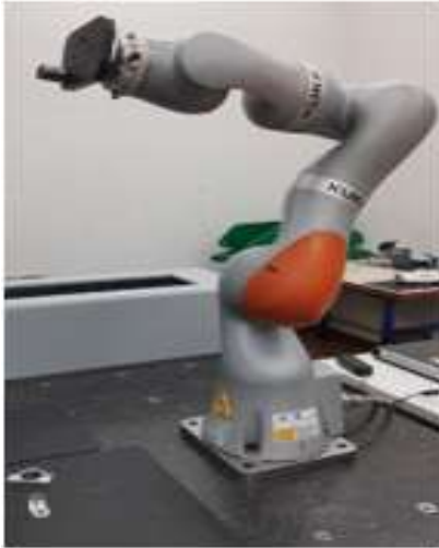
Fig. 1. Real reference system, KUKA iiwa robot with camera attached to the end effector and parts arranged on a work area.
