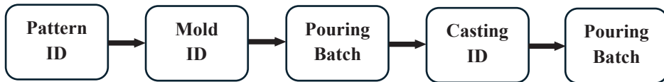
Fig. 2. Traceability chain linking Pattern ID, Mold ID, Pouring Batch and Casting ID
