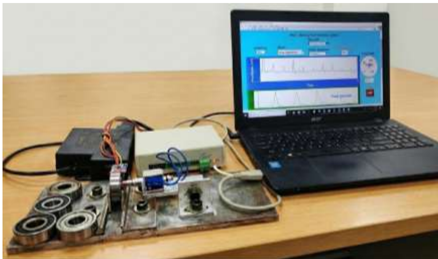
Fig.9 LabVIEW controlled PSoC embedded test bench for bearing fault detection system
