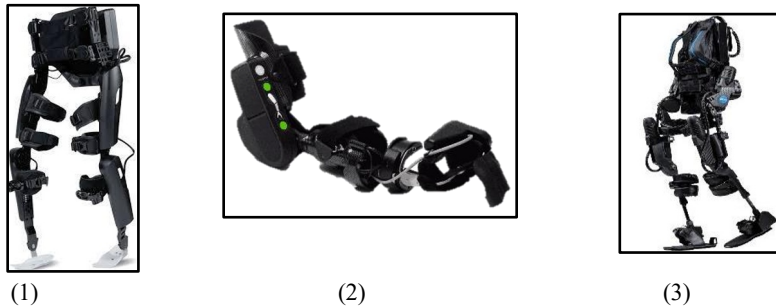
Fig. 2. Exoskeletons categorized based on limb coverage 1. ReWalk (lower-limb) [5], 2. MyoPro Hand Brace (upper-limb) [14] 3. EksoGT (lower-limb) [6]
