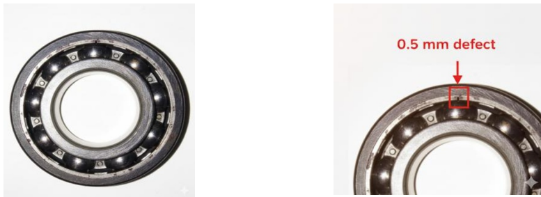
Fig. 1. Outer race fault in the SKF6206 Bearing with a 0.5 mm defect.
