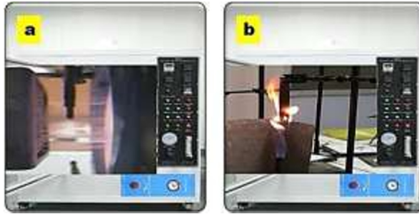
Fig. 2. UL-94 Vertical burning of hybrid composite specimen (a) Before burning; (b) After burning.
