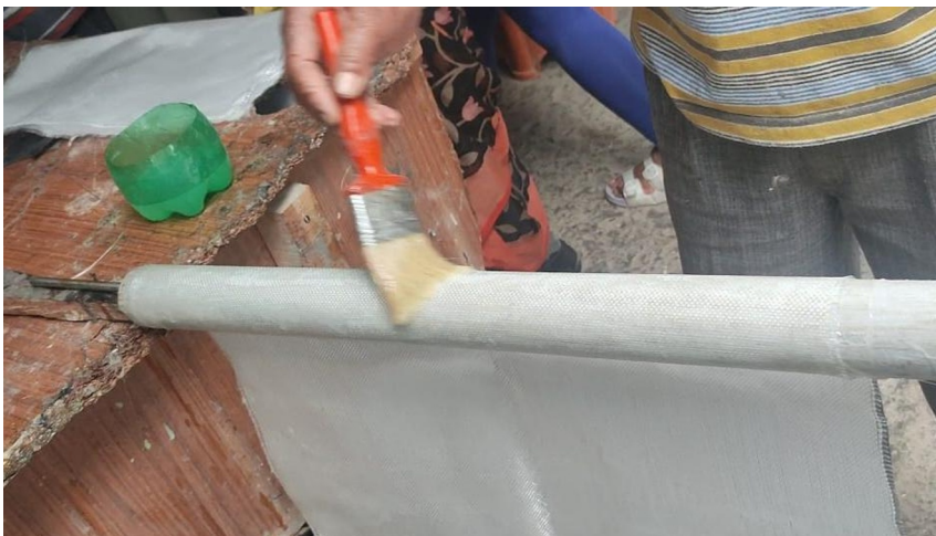
Fig. 1. Hand layup process of thin cylinder.
