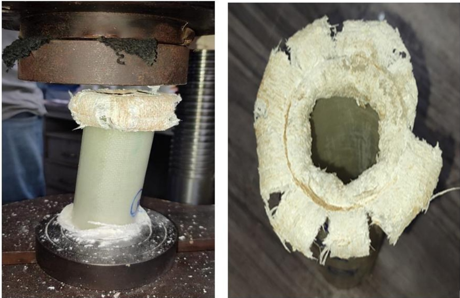
Fig. 3. Progressive failure of composite shell during compression test.
