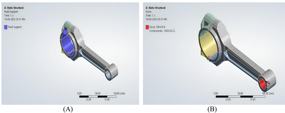
Fig 3. Boundary Conditions, (A) fixed support applied at the big end, (B) axial force applied at the small end
