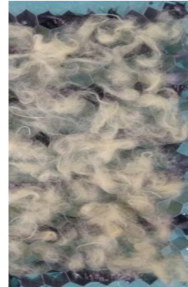
(Honeycomb Core with Kevlar interface)
