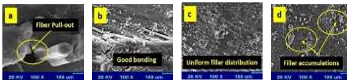
Fig. 5 Microstructural analysis of hybrid composites after tensile testing
