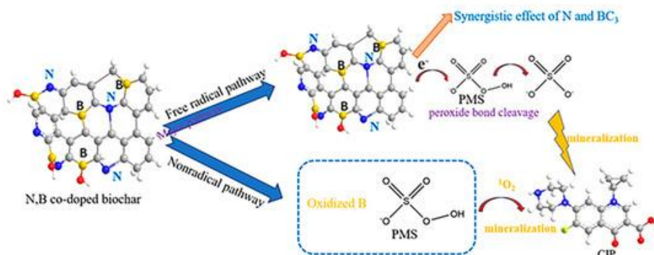
Fig. 3. Illustration of the degradation mechanism for Ciprofloxacin (CIP) by N, B co-doped biochar. [13]
