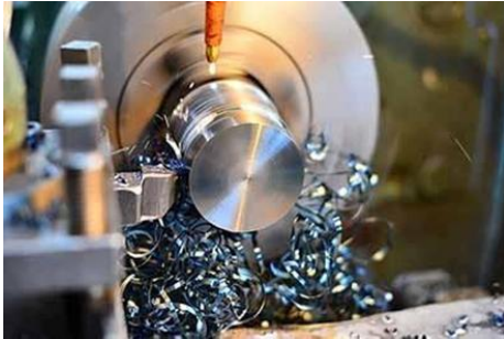
Fig. 1. Chip formation During Machining [1]
