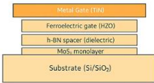
Fig. 1. Schematic cross-section of MoS 2 -based GFNCFET showing layer stack: Metal Gate (TiN), Ferroelectric gate (HZO), h-BN spacer, MoS 2 monolayer, and Substrate (Si/SiO 2 )
