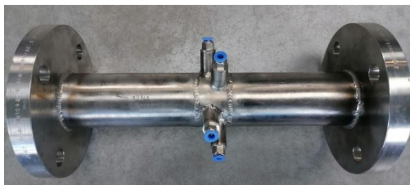
Fig. 4. View of the measurement module with the welded ISA 1932 nozzle.
