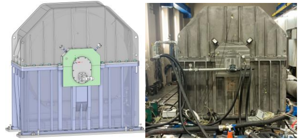
Fig. 3. 3D model of the flywheel and finished product.
