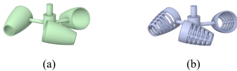
Fig. 2. Geometry of the tested impellers: Jet-1 (a), Jet-2 (b).
