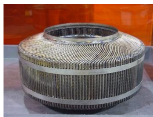
Fig. 2 CWPSR applied on Capstone C30 [24]
