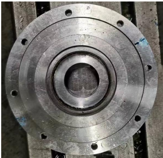
Figure 14 End cover equipped with brush seal
