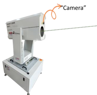
Figure 1. Lidar equipment with attached camera used for observation (MK-SMART 1)
