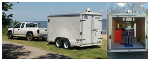
Figure 1. University of Virginia Wind Observatory on Wheels (UWOW). The Doppler Wind Lidar is installed on a mechanically-operated lift table in a cargo trailer.
