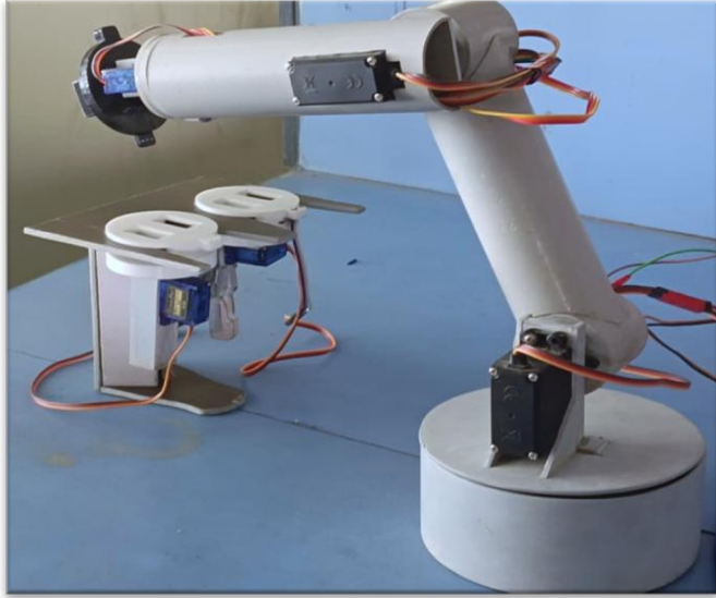
Fig. 4. Robotic arm with both Mechanical gripper and Magnetic separator
