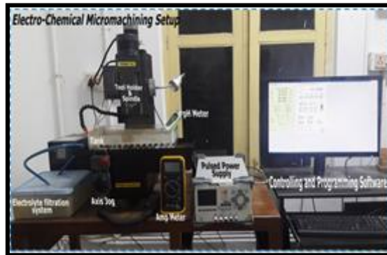
Fig. 1. Electrochemical micromachining station used for micro ECM drilling
