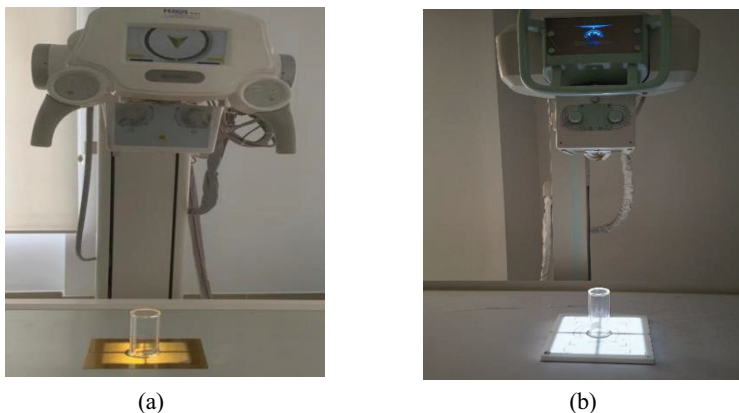
Fig. 1. collimator test tool and beam alignment tool (a); Leeds Test Objects' FLUORO-4 phantom and beam alignment tool (b)
